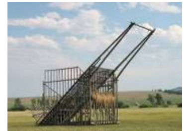
The beaverslide haystacker revolutionized haying when it was invented in the Big Hole Valley a century ago. Still in use, the beaverslide pictured above is located near Nevada Creek in Powell County.
